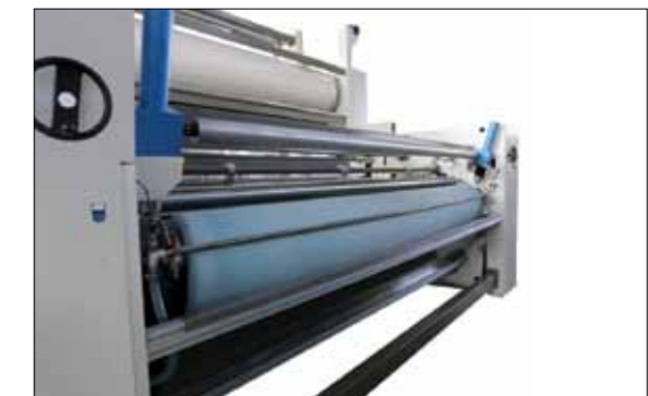
High efficiency compressive shrinking machine with grinding device including cooling water distributor and tensionless synchronization.
