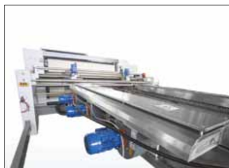
Stenter frame entirely made in stainless steel. The conical and parallel fields allow an optimal control of the width all along the machine.
