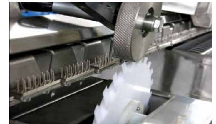
The patented pneumatic system allows to pin the minimum quantity of fabric on the chain.
