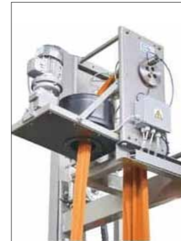
The automatic rope detwister, allows an easy and fast pass to avoid excessive tensions in the fabric.
