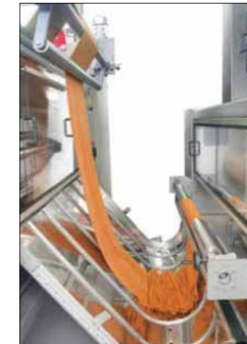
The 4T version comes with a J-BOX between squeezing and impregnation foulards. The system includes a tension control system with an automatic compensation roller.
