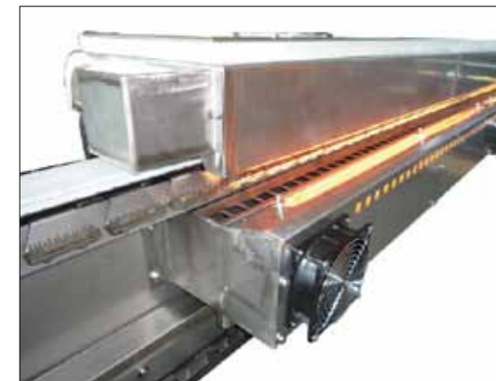
High efficiency drying system for the selvedges. Composed by circulating hot air and infrared resistances.
