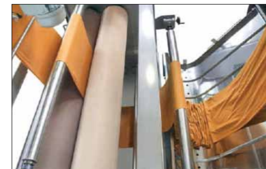
The heart of the machine is represented by its squeezing rollers, covered by special rubber. Squeezing pressure is programmed by the operator through the touch screen.
