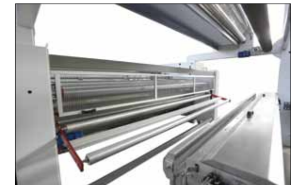
Non-stop combined A-frame, rolling up device and plater with adjustable folding waves.
