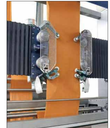
The exit system composed by the patented magnetic stretcher to control fabric's width and adjustable folder. The stretcher allows to minimize the tensions of the fabric by overfeeding it.
