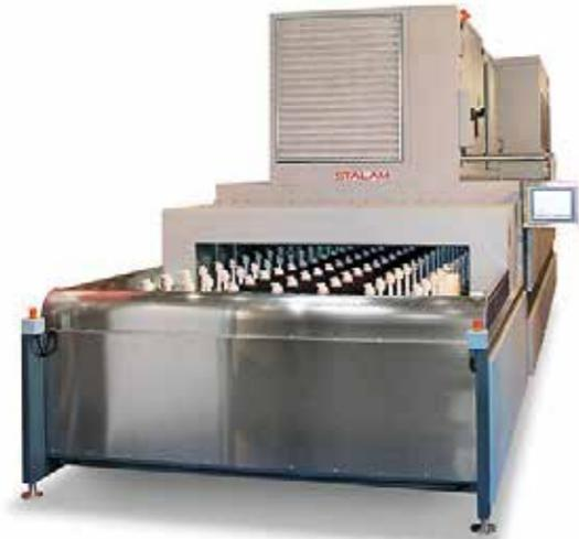
The air forced through the product is heated up to the desired temperature without using any external (additional) energy source by recovering the heat dissipated by the RF generator. Both the RF energy and the warm air forced through the product contribute to water evaporation. This combined process, other than being extremely efficient, enables a precise control of the product's internal temperature, thus optimising the drying quality results.
