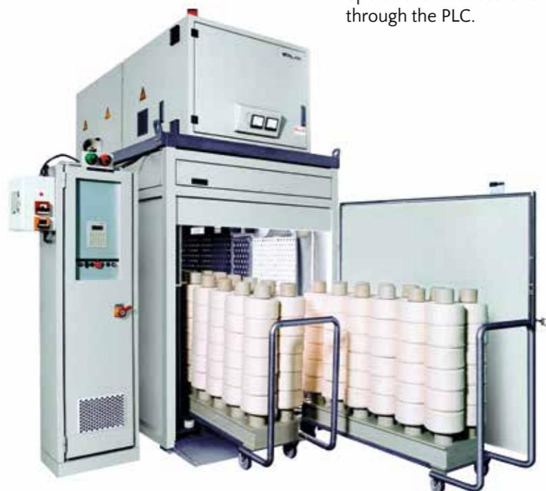
TCRF dryers with 1 or 2 trolleys specifically designed for yarn packages, and a dryer model with 2 trolleys suitable for both tops and packages, are available.
