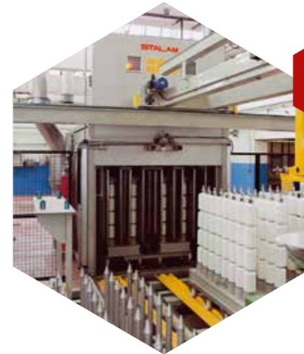
The TCRF (Thermo-Controlled Radio Frequency) model dryers represent the outcome of the researches carried out by STALAM in co-operation with Messrs. Loris Bellini as to the drying of yarn packages and tops in bobbin or bump form by means of a combination of RF energy and forced air circulation. They can surely be considered as the most sophisticated batch-type textile dryers available worldwide.
