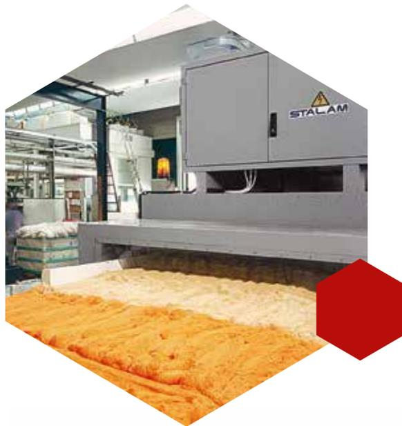
The *LTRF* (Low Temperature Radio Frequency) series dryers are especially designed for the low temperature drying of all "loose" textile products.
