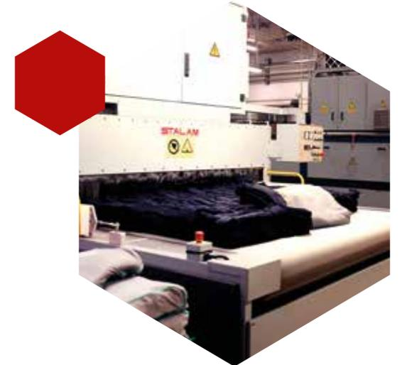
The RF/T series dryer can be considered the only industrial Radio Frequency drying equipment specifically designed for the tensionless drying - partial or complete - of woven or knitted fabrics.
