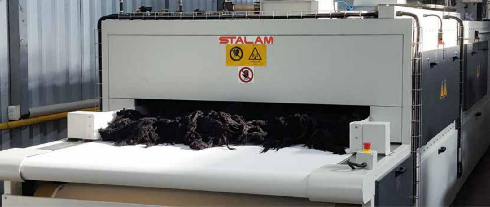
The *RFA/S COMBO* series dryers are the latest evolution of the RF and forced-air circulation combined drying equipment developed by STALAM in the early nineties.
