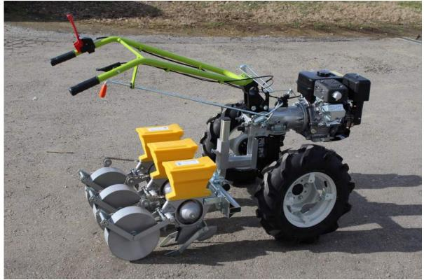
The *SM Seeder* is a modular seeder: the number of sowing elements varies from 1 to 4 according to the customer's needs. The sowing elements are applied behind a cultivator or a motor hoe and it is possible to sow vegetables, cereals, legumes, officinal and aromatic herbs, both with naked or pillolated seeds.
