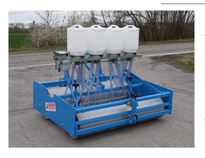
In the *electronic system*, the movement of the sponge is transmitted by a 12 V electric motor: by varying the speed of this motor with a convenient control, you can adjust the quantity of seed coming out. It is possible to sow from 1 to 1000 kg / Ha. This model is more precise as regards calibration, it allows you to program the dosage even if you change the type of seed. However, more attention is needed in programming the machine and specialized personnel is required.
